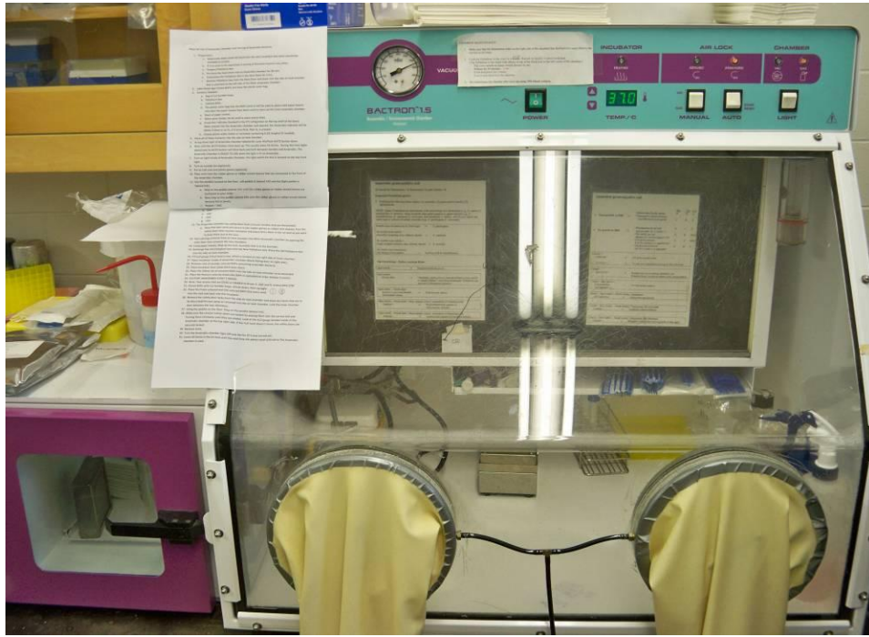
Figure 1. Anaerobic Chamber – Anaerobic microorganisms were incubated in this Bactron 1.5 Anaerobic Environmental Chamber (Sheldon Labs, Crystal Springs, MS).
